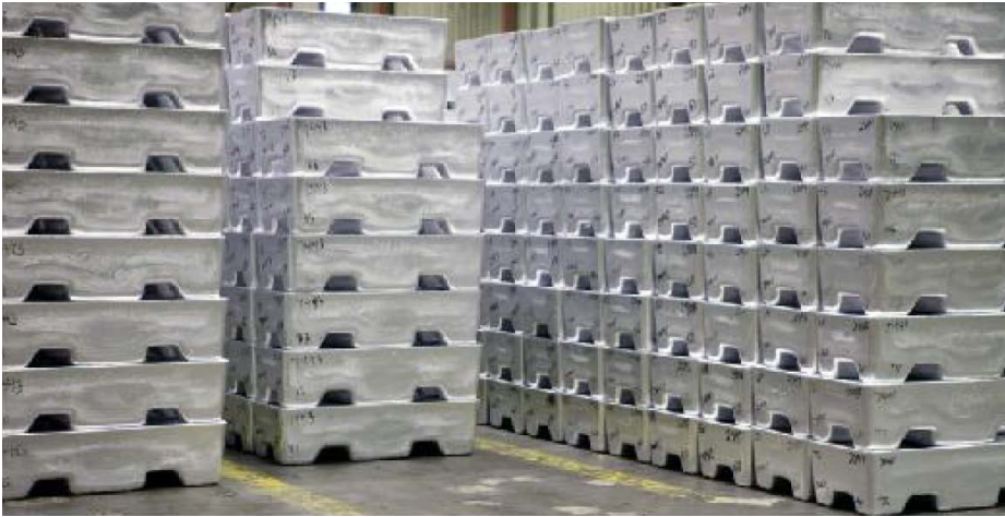
Stacks of Zinc Alloy Jumbos per ASTM B852, Standard Specification for Continuous Galvanizing Grade (CGG) Zinc Alloys for Hot-Dip Galvanizing of Sheet Steel, and B897, Standard Specification for Configuration of Zinc and Zinc Alloy Jumbo, Block, Half Block, and Slab Ingot. Image courtesy of Teck Metals Ltd. www.teck.com
