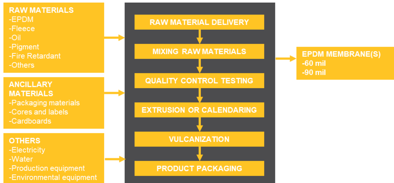
Figure 1: VersiGard® Non-Reinforced EPDM production process map
