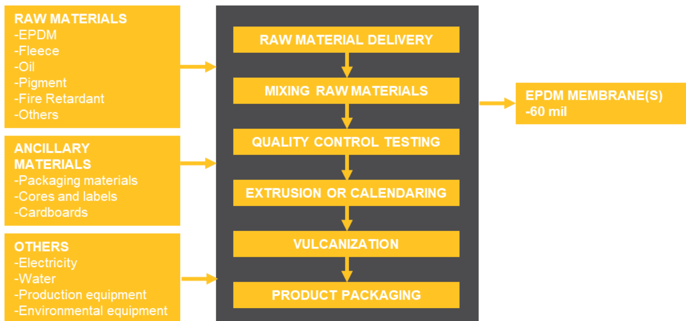
Figure 1: VersiGard® White Reinforced EPDM production process map
