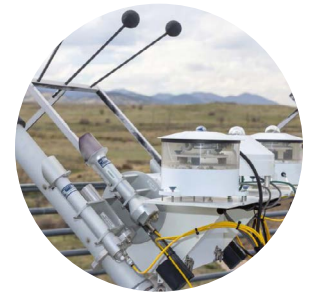
Device used to measure various types of irradiance, per E816, E824, G130, G207
