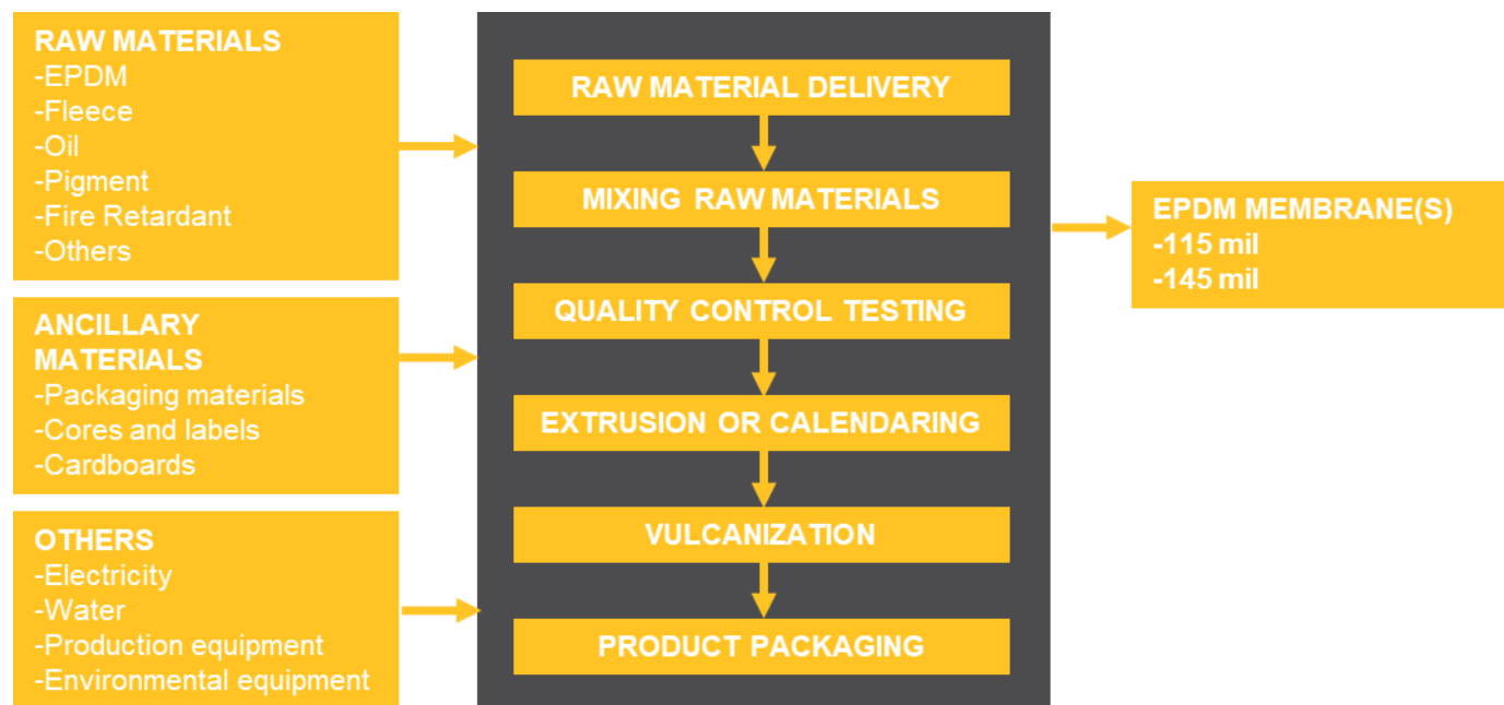
Figure 1: VersiFleece White EPDM production process map
