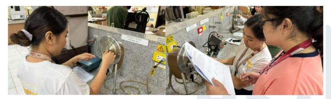
Standards used: ASTM D5342 Standard Test Method for Resistance to Bending of Paper and Paperboard
