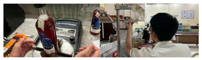
Standards used: ASTM D3198 Standard Test Method for Application and Removal Torque of Threaded or Lug-Style Closures and ASTM D1709 Impact Resistance of Plastic Film by the Free-Falling Dart Method
