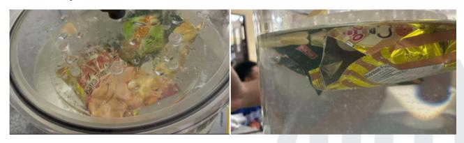
Standards used: ASTM D3078 – Standard Test Method for Determination of Leaks in Flexible Packaging by Bubble Emission
