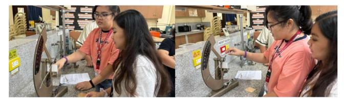
Standards used: ASTM D3689 Internal Tearing Resistance of Paper
