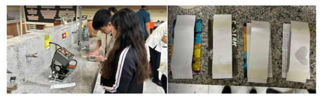
Standards used: ASTM D5264 Standard Practice for Abrasion Resistance of Printed Materials by the Sutherland Rub Tester
