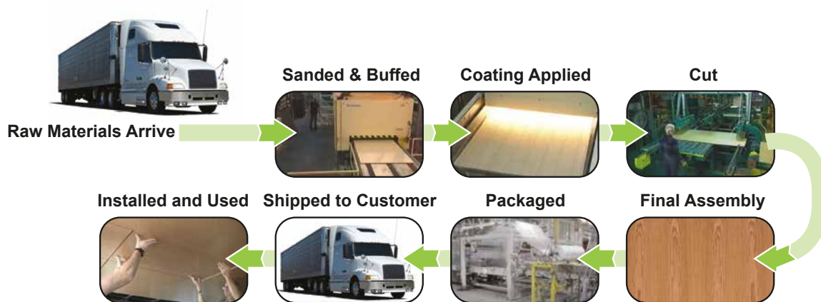
Figure 3. Process for manufacturing Woodworks Solid Wood Ceiling and Wall Products
