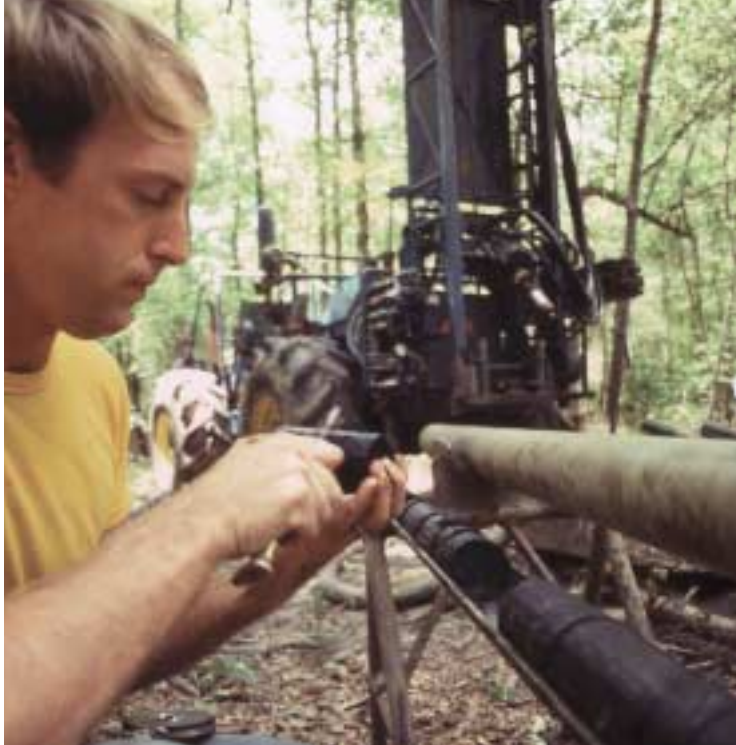
Figure 3 — Standardization of coal core sampling practices (left) provide a more versatile, consistent, and cost-effective method of sampling (D 5192). Prior to this, the only sanctioned method of sampling for determination of coal rank (D 388) was by face channel samples from mines or test pits (above).
