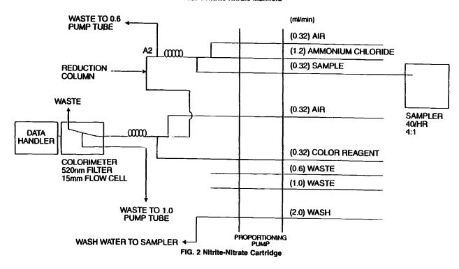
Note 3-A pump tube with 0.081-in. (2.1-mm) inside diameter can be used in place of the 2-mm glass tube.
