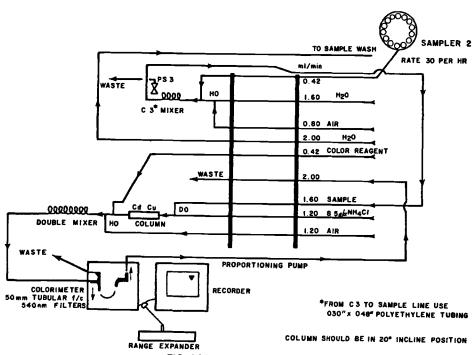
FIG. 1 Nitrite-Nitrate Manifold
