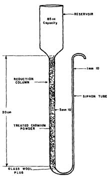
FIG. 3 Cadmium Reduction Column
