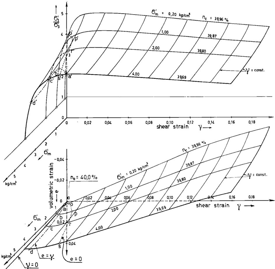
FIG. 9—Stress-Strain Surfaces for a Dense Sand.
