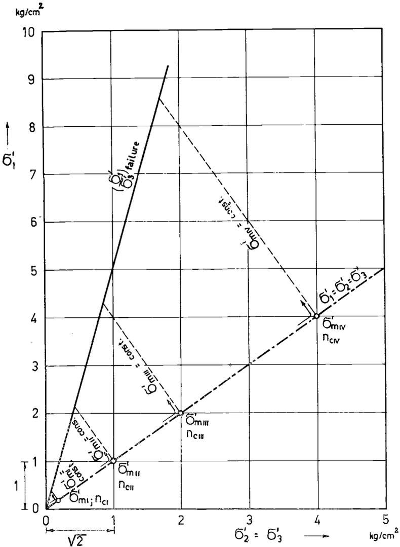
FIG. 8—Loading Paths for Drained, Effective Mean Normal Stress Constant Tests.
