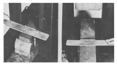
FIG. 12 Method for Alignment of Specimen
