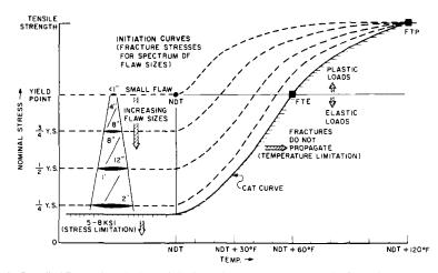
FIG. 1 Generalized Fracture Analysis Diagram Indicating the Approximate Range of Flaw Sizes Required for Fracture Initiation at Various Levels of Nominal Stress, as Referenced by the NDT Temperature<sup>6,7</sup>
