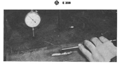
FIG. 8 Notching of Crack-Starter Weld Deposit
