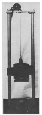
FIG. 5 Portable Drop-Weight Test Machine Used for Tests at Different Fabrication Sites
