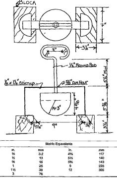
FIG. 1 Ball-drop Apparatus
