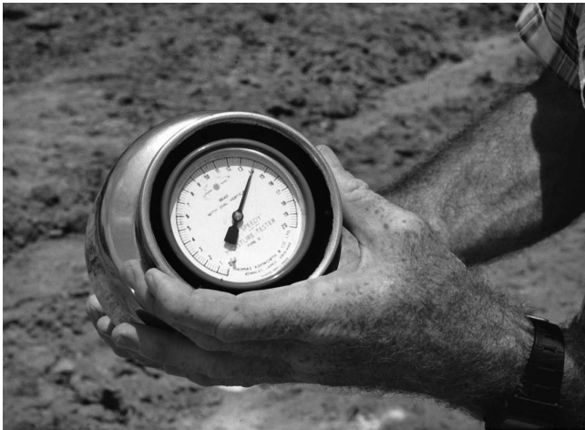
Fig. 11C—Calcium carbide gas pressure tester method (ASTM D4944).
