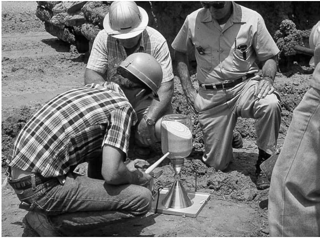
Fig. 5C—Sand cone method (ASTM D1556).
