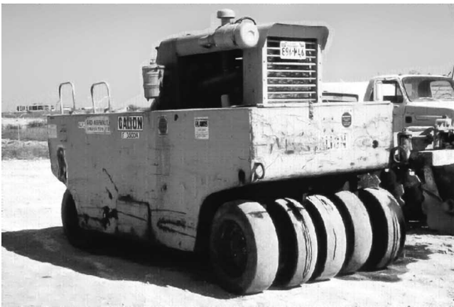
Fig. 3C —Pneumatic roller—provides static rolling for soils of low to no plasticity.
