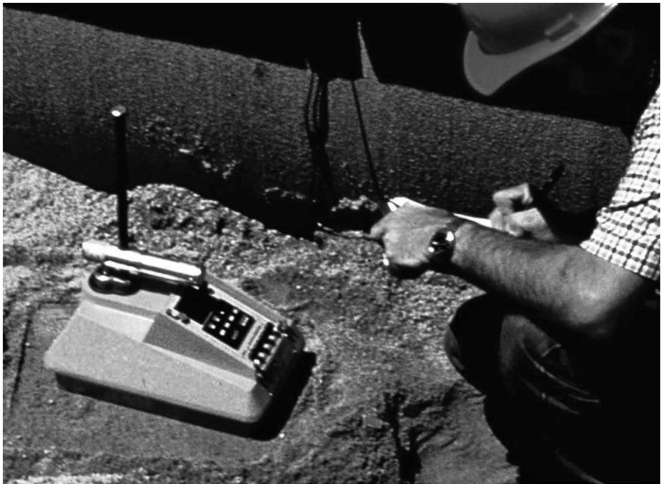
Fig. 9C—Nuclear method (ASTM D6938).
