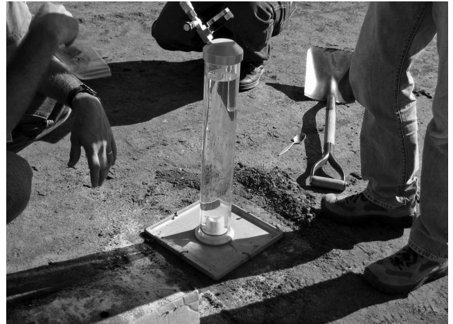
Fig. 6C—Rubber balloon method (ASTM D2167).
