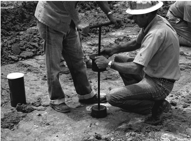
Fig. 7C—Drive cylinder method (ASTM D2937).
