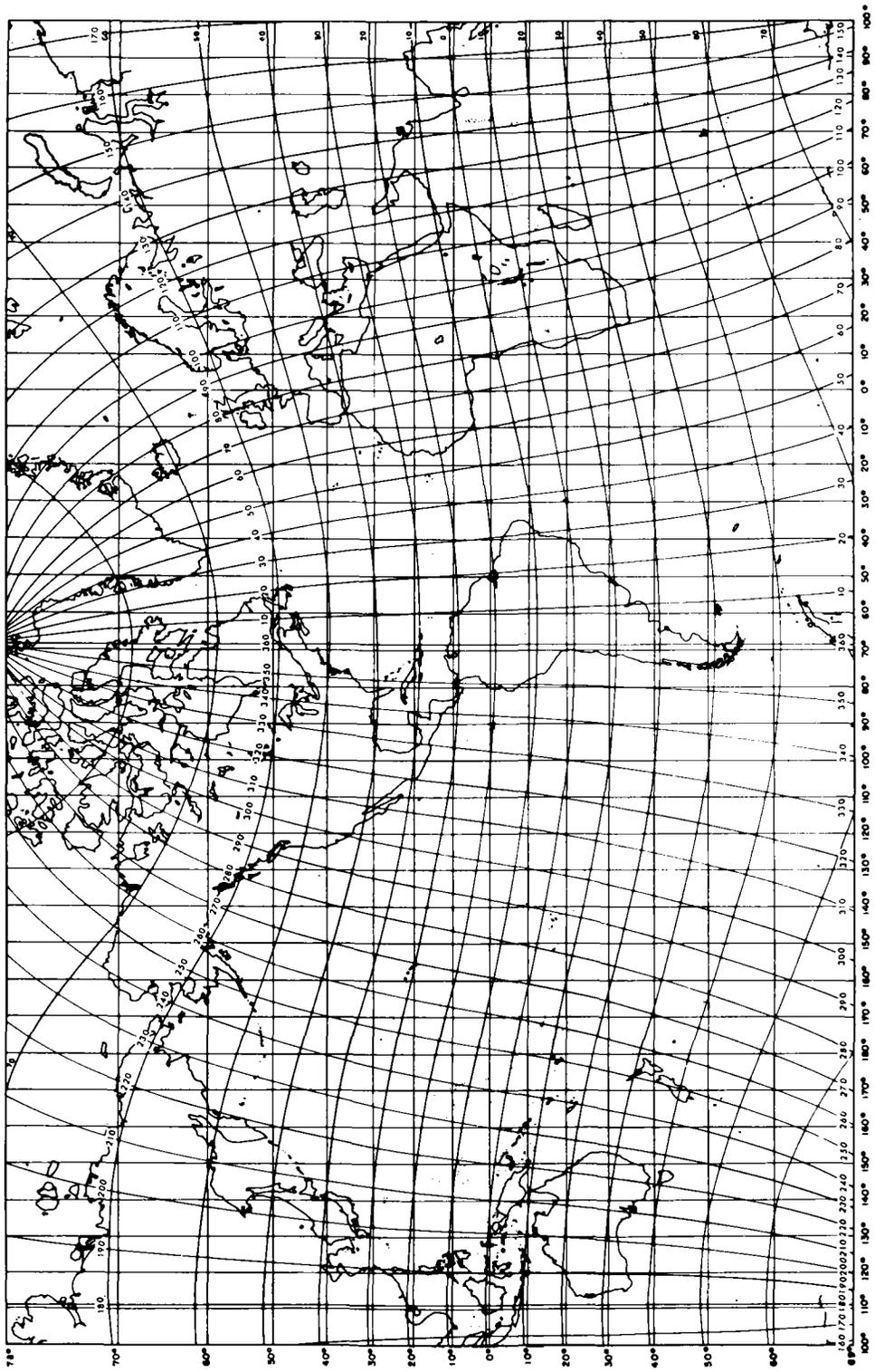
FIG. 33.—Geomagnetic Dipole Field Coordinate Grid (Curved Lines) Superimposed on a Mercator Projection of the Earth. (From reference (11) of Appendix I.)
