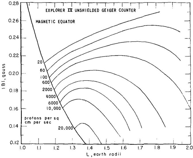
FIG. 35.—Contours of Constant Proton Flux ( $E > 31$  Mev) in B and L Coordinates. These data correspond to those of Fig. 29. (From reference (13) of Appendix I or reference (27) of Part II.)
