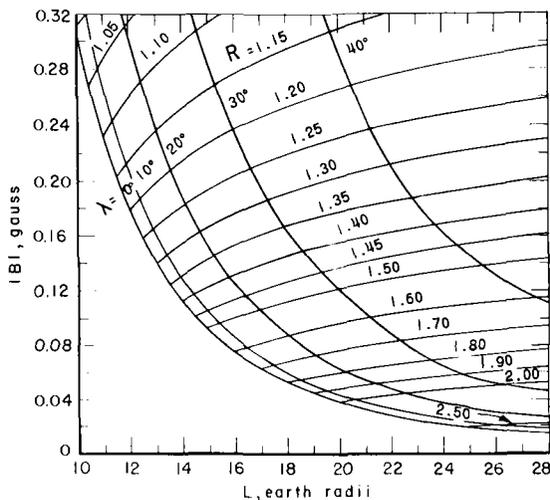
FIG. 34.—Centered Dipole Coordinates Defining  $B$  and  $L$ . (From reference (13) of Appendix I or reference (27) of Part II.)
