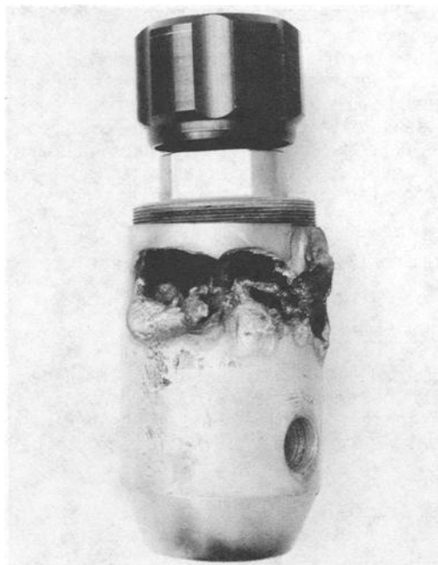
Fig. 5 - Example of a regulator ignited by adiabatic compression test - Aluminum body
