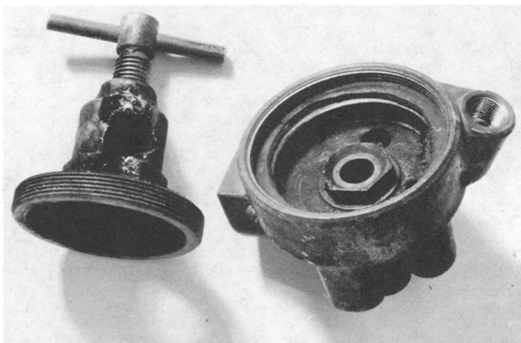
Fig. 6 - Ignition with a brass body regulator
