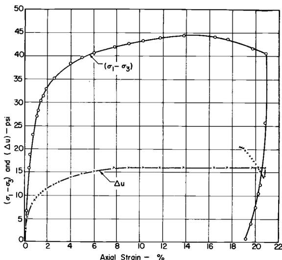
FIG. 10—Typical Stress-Strain Curves for Overconsolidated Specimens of Kaolinite.
