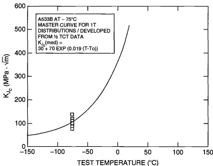
Note 1—Toughness data are converted to 1T equivalence.
