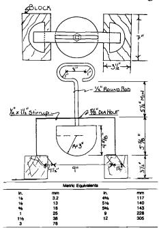
FIG. 1 Bail-drop Apparatus
