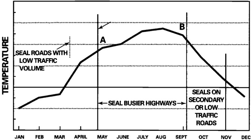
FIG. D3—Recommended seal coat program based on annual thermal cycle.
