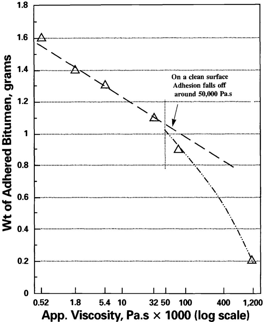
FIG. D1—Viscosity of binder versus adhesion of binder to aggregate surface.
