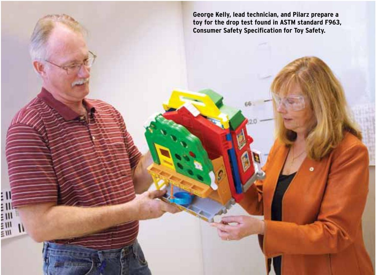
**George Kelly, lead technician, and Pilarz prepare a toy for the drop test found in ASTM standard F963, Consumer Safety Specification for Toy Safety.**
