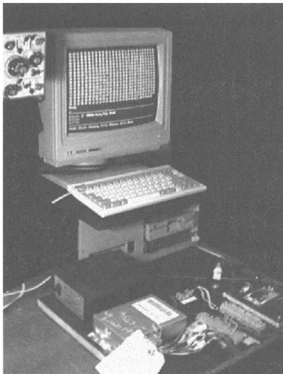
**FIG. P.4—Laboratory download of an SRS ECU.**
