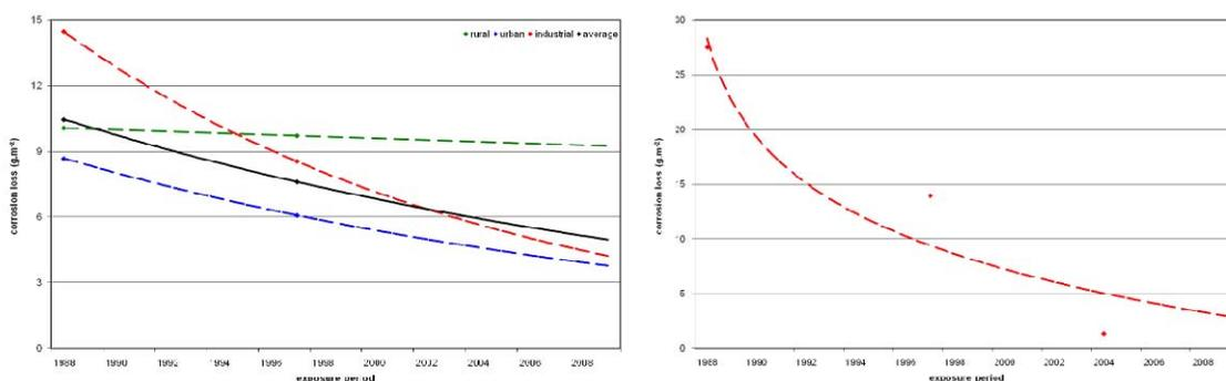
**Figure 7:** Yearly corrosion loss of copper decreasing at European test sites (ICP program) and at Czech industrial test site Kopisty (No 03)
