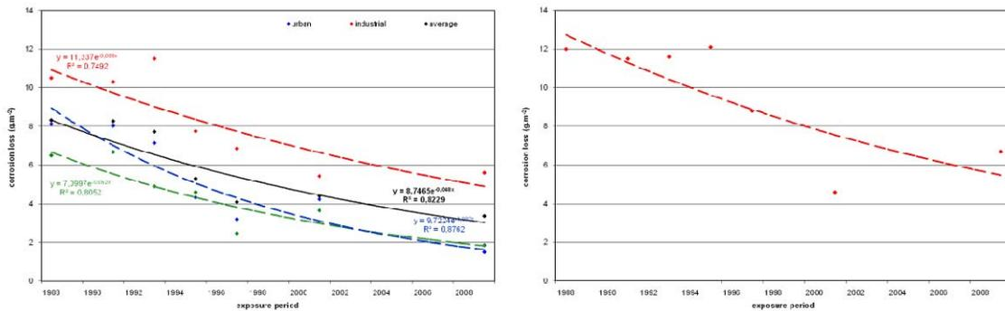
**Figure 5:** Yearly corrosion loss of zinc decreasing at European test sites (ICP program) and at Czech industrial test site Kopisty (No 03)
