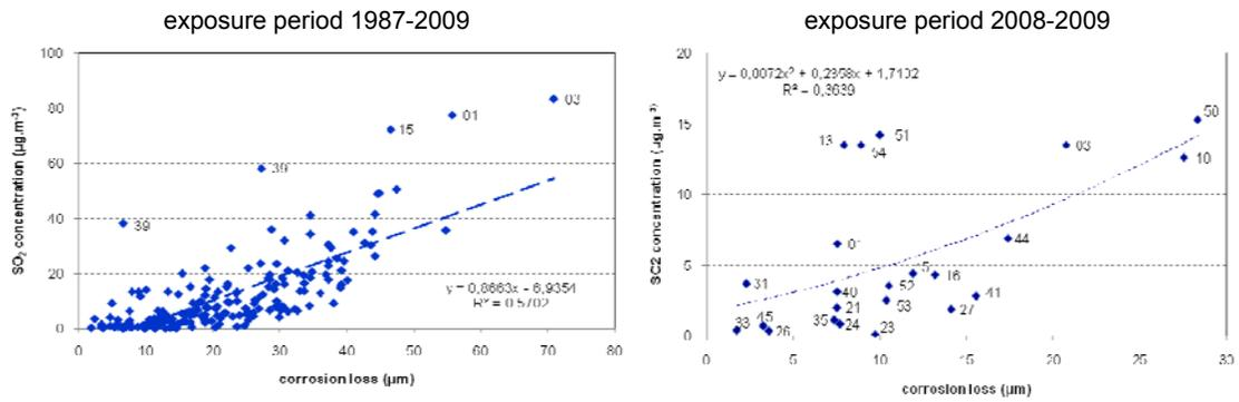
**Figure 4:** The plot of SO<sub>2</sub> concentration and yearly corrosion loss of carbon steel (all test sites)
