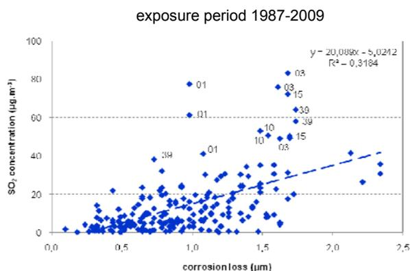
**Figure 6:** The plot of SO<sub>2</sub> concentration and yearly corrosion loss of zinc (all test sites)
