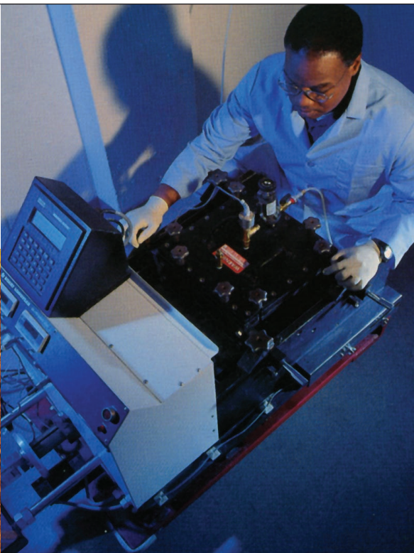
Direct Shear (Interface Friction) Testing ASTM D5321
