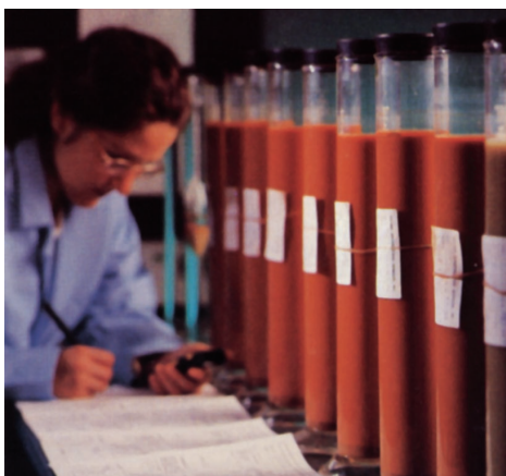
Grain Size Analysis ASTM D422
