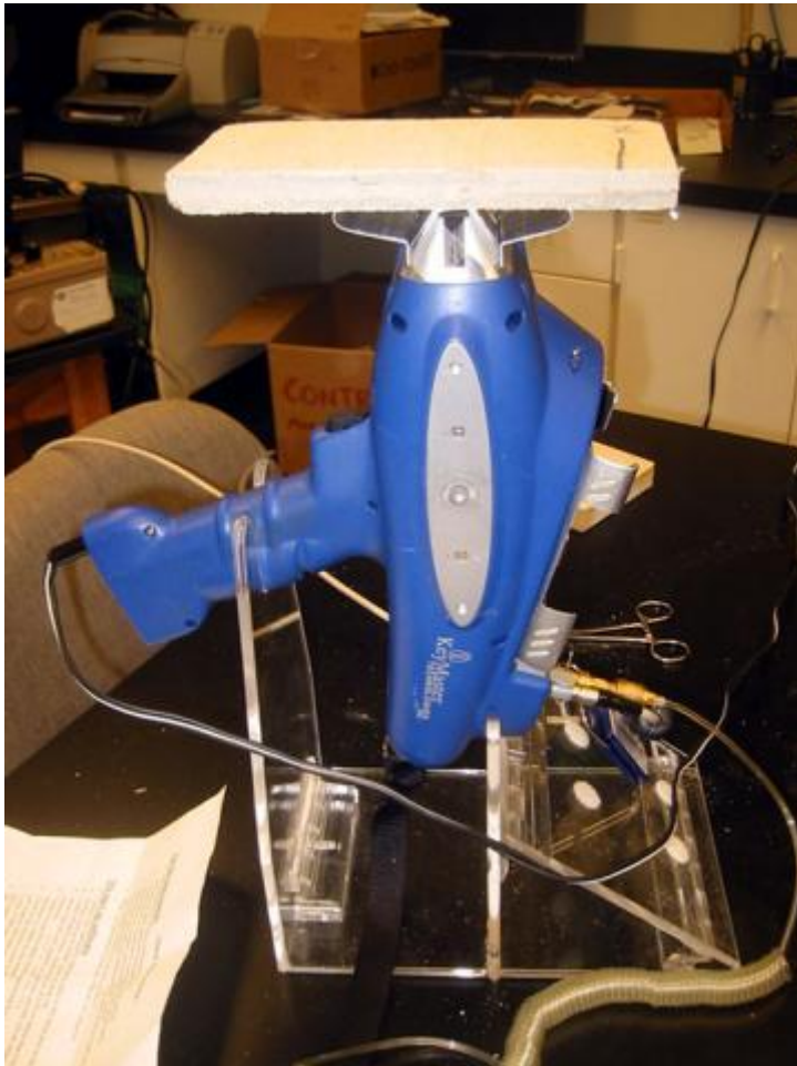
XRF unit and ceiling tiles (with vacuum system in place for low atomic # detection)
