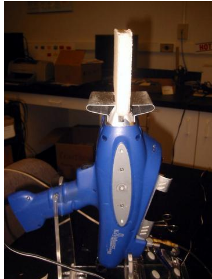
XRF unit and ceiling tiles (with vacuum system in place for low atomic # detection)
