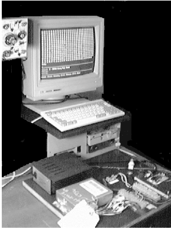
FIG. P.4—Laboratory download of an SRS ECU.
